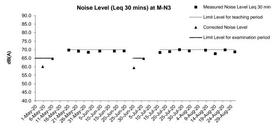
Remark: Corrected Noise Level was applied on 5, 11 May 2020, 30 June 2020 and 6 July 2020; Corrected Noise Level = 10\* log(10^(Measured Noise Level/10) – 10^(Baseline Noise Level/10))
